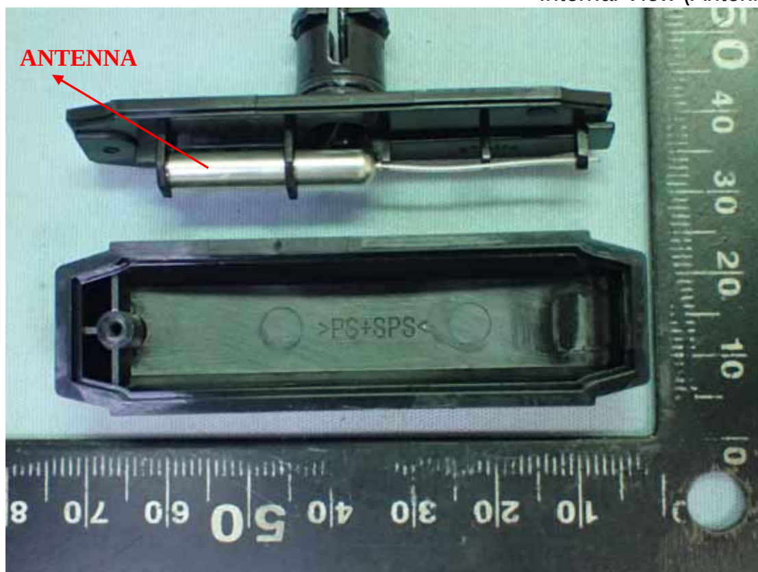
Figure 20 Internal View (Antenna View)
