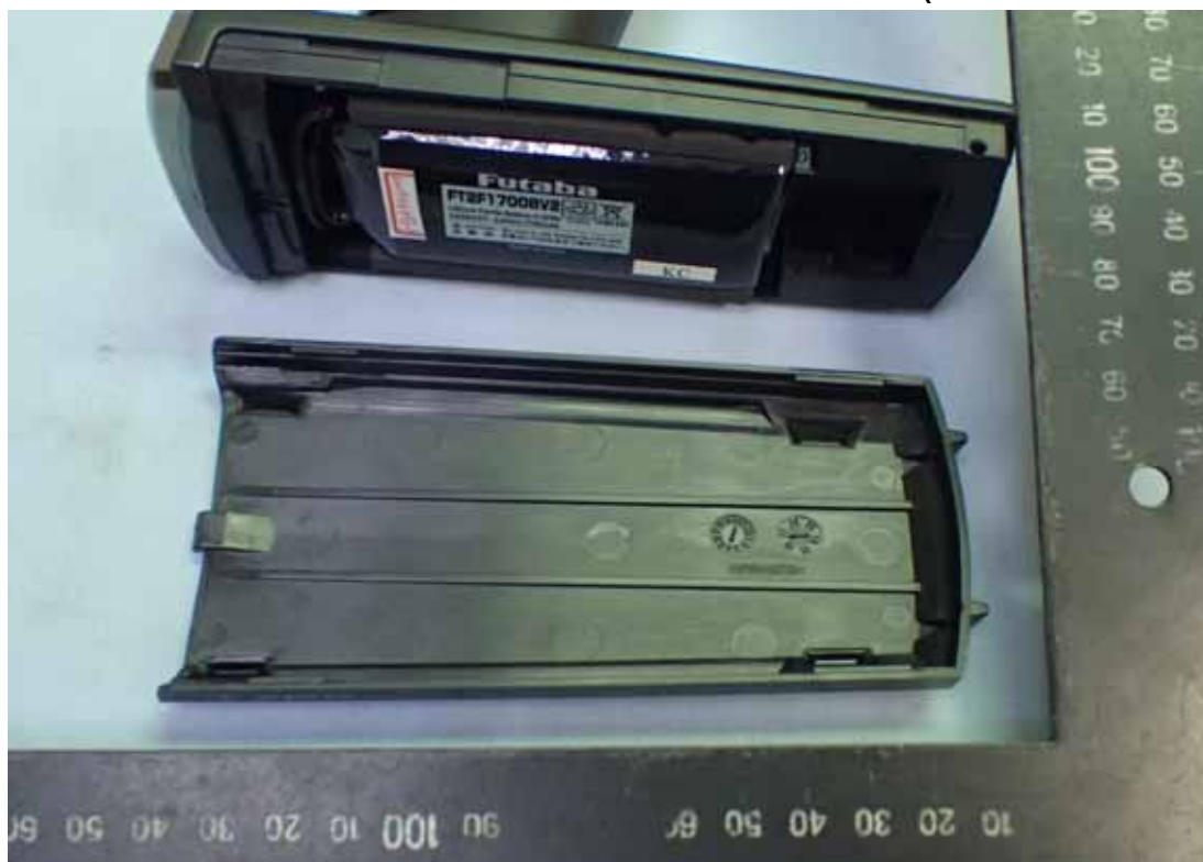
Figure 7 Internal View (Battery)
