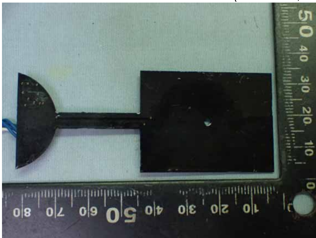
Figure 18 Internal View (NFC Antenna, Back View)
