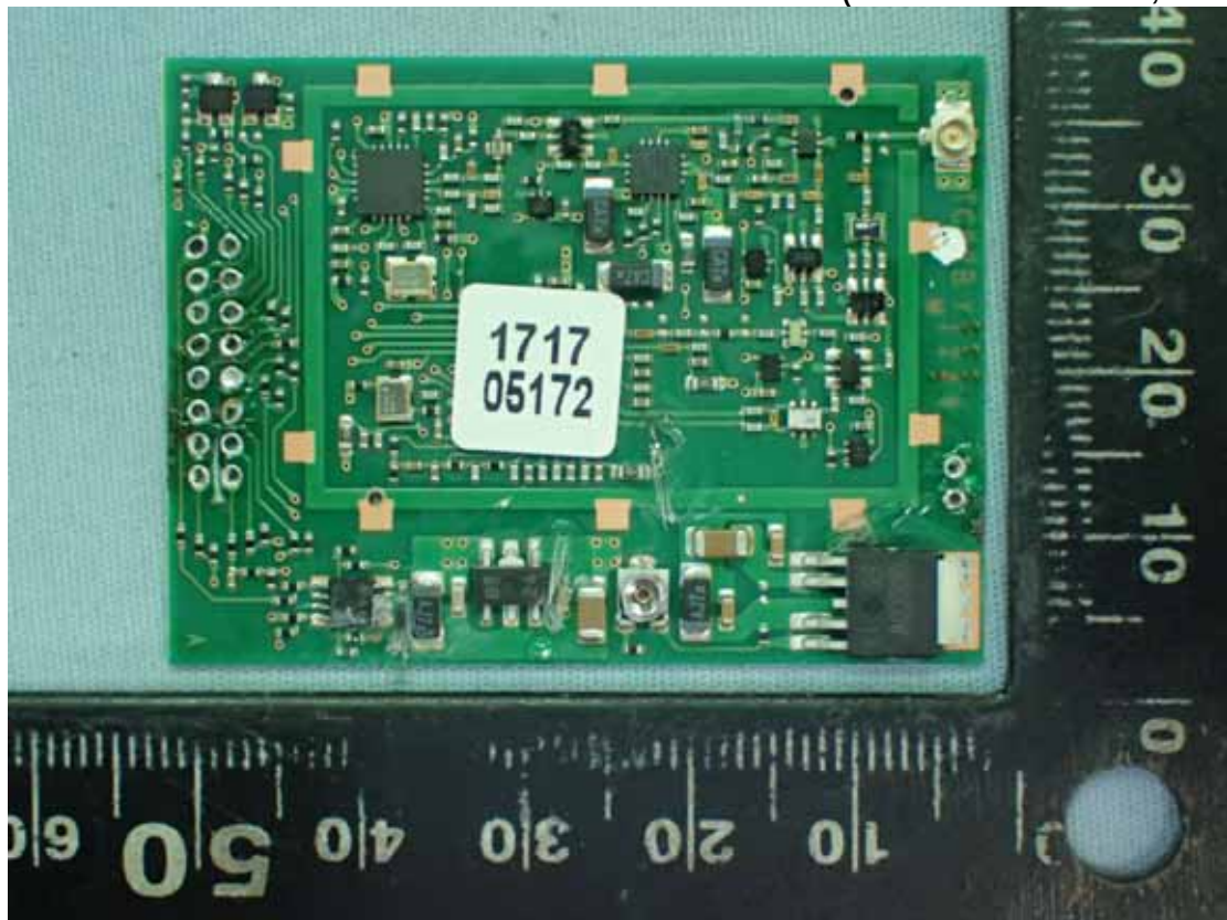
Figure 44 Internal View (RF Control Board, Front View)
