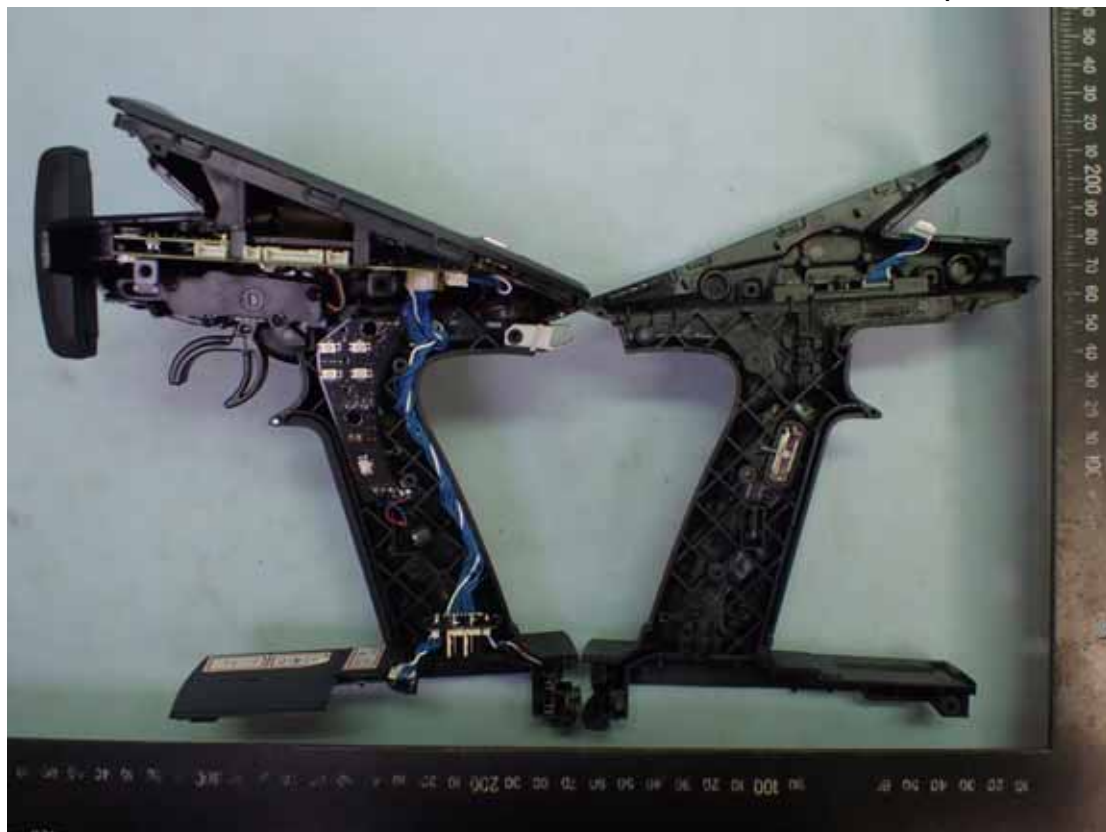
Figure 8 Internal View (Removed Covers)
