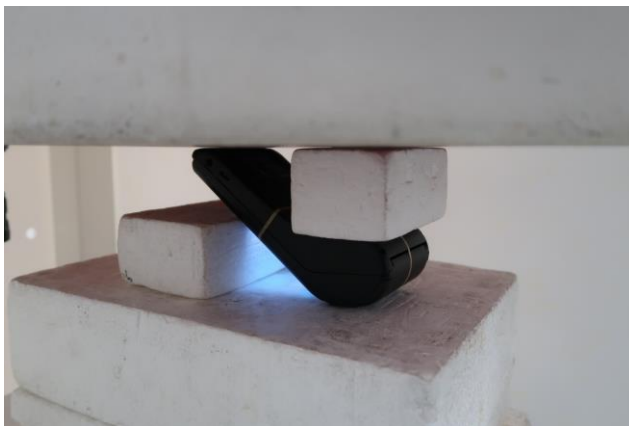
Rear Slant, Test Separation 0 mm
