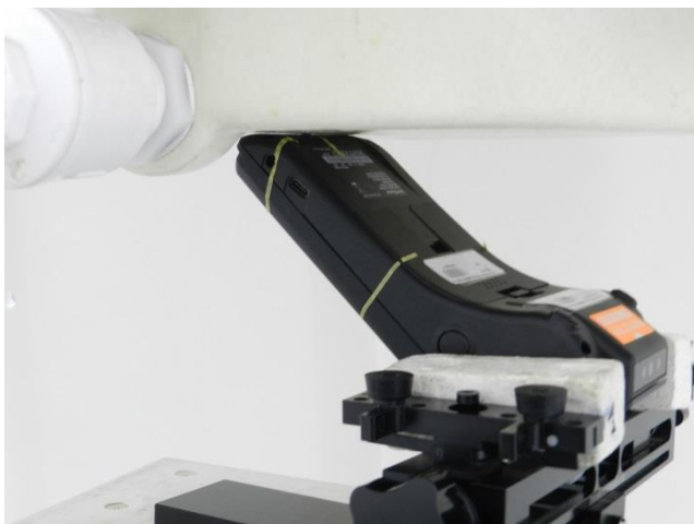
Rear Slant, Test Separation 0 mm
