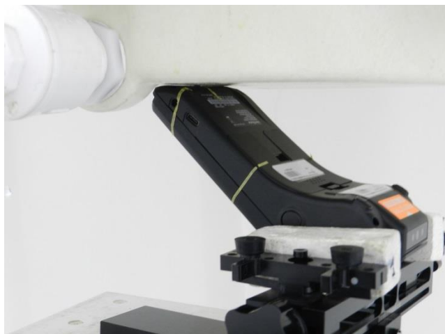
Rear Slant, Test Separation 0 mm
