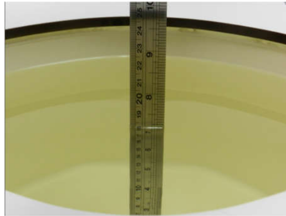
Fig 10.1 Photo of Liquid Height for Body SAR
