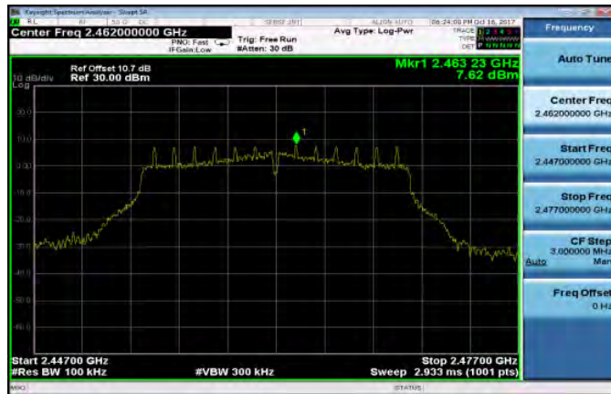
802.11n_HT20 PSD FOR BANDEDGE LIMIT (CH-Low)
