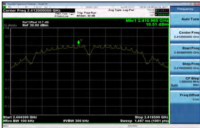
802.11b PSD FOR BANDEDGE LIMIT (CH-High)
