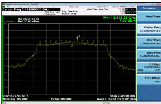
802.11g PSD FOR BANDEDGE LIMIT (CH-Low)
