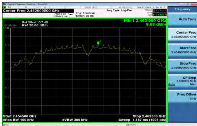
802.11g PSD FOR BANDEDGE LIMIT (CH-Low)
