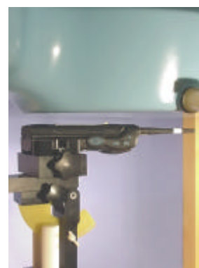
Body-worn SAR Test Setup with 1.5cm separation distance
