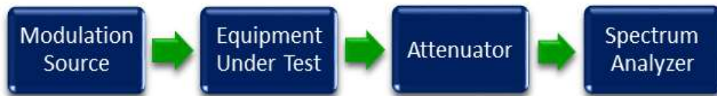
Figure 3: Occupied Bandwidth Test Setup
