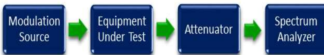
Figure 2: Modulation Characteristics Bandwidth Test Setup
