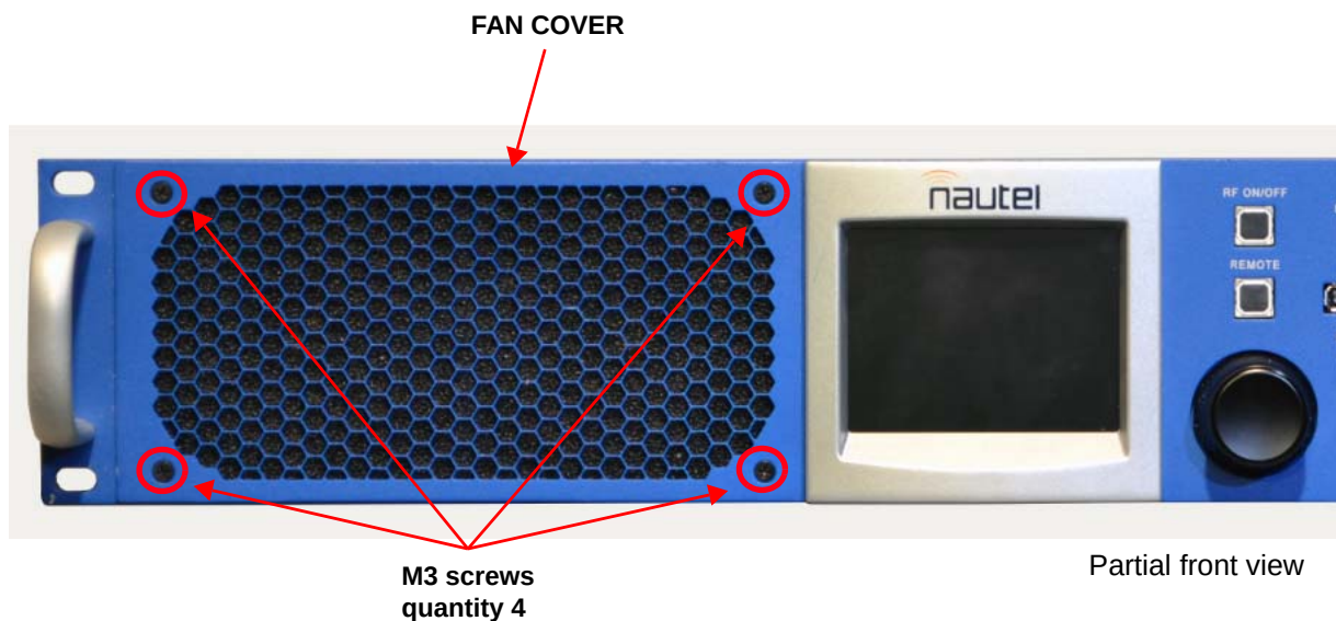
Figure 2.3.1: Replacing Air Filter
