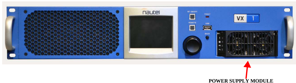
Figure 3.1.6: Location of Power Supply Module
