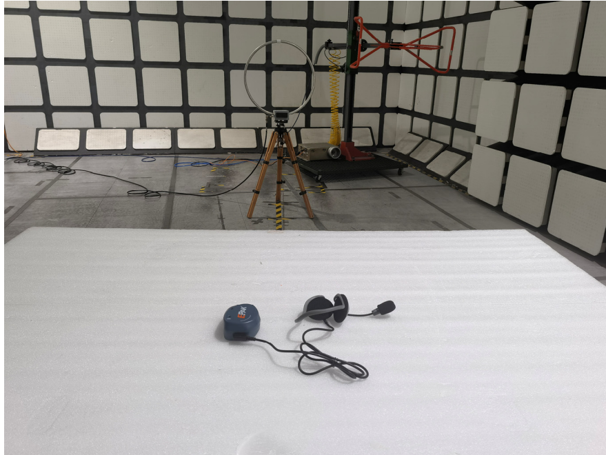
Radiated Emissions View (Below 30MHz)
