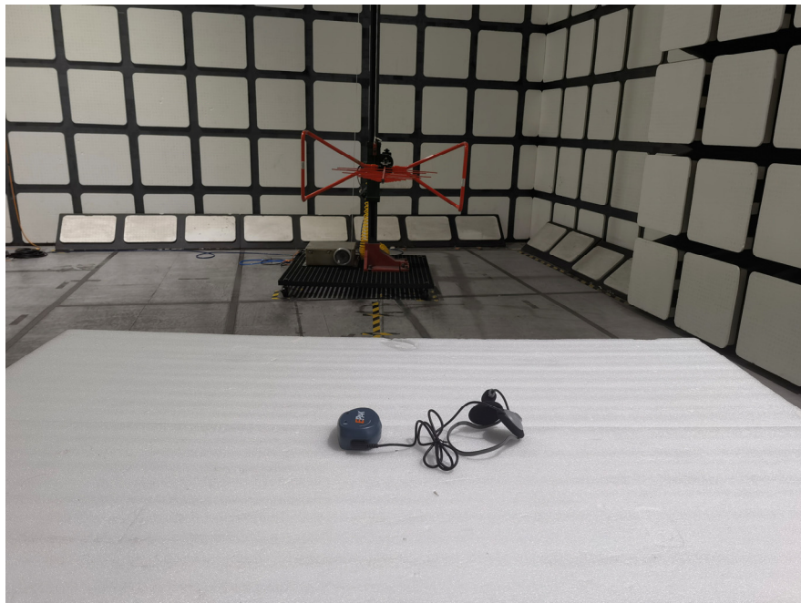
Radiated Emissions View (Below 1 GHz)
