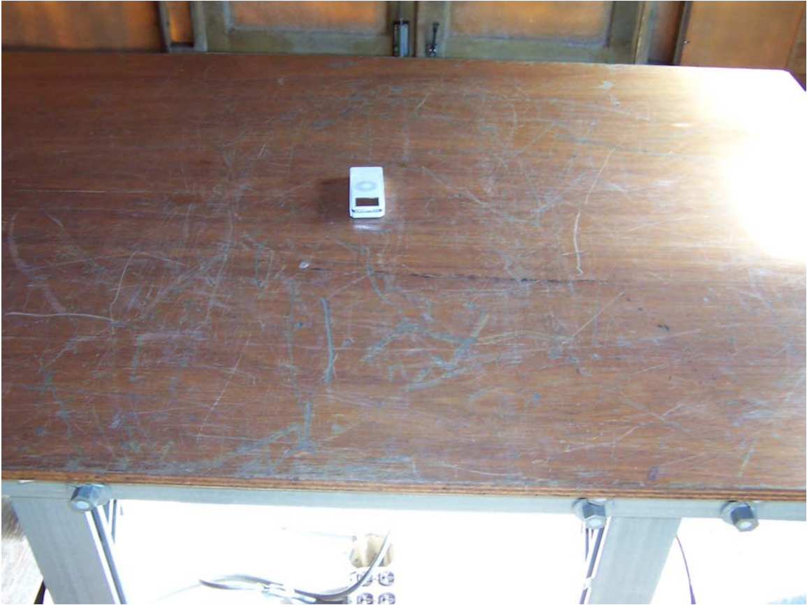
Radiated Emissions Test Setup (X-axis)
