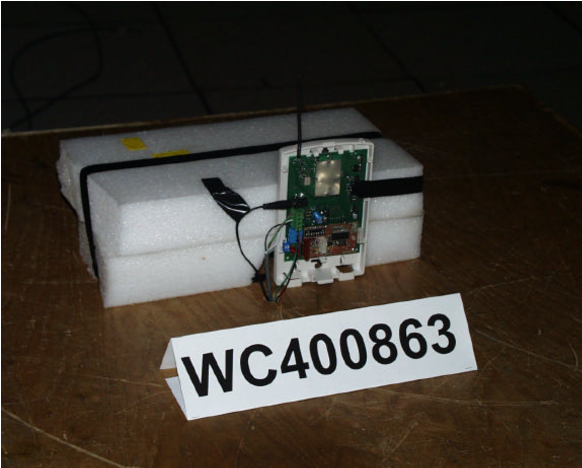
Figure 1: Picture of DUT on test table, showing daughterboard connected and bus wires for each of the security panels connected.
