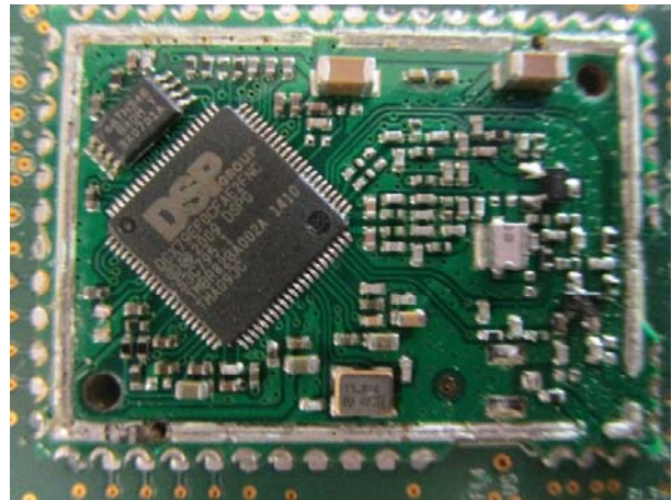
RF Module Cover Off View
