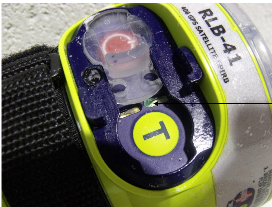
Corrosion on water contacts
