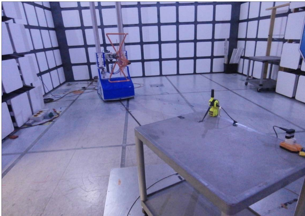
Figure 8 - Test Setup - < 1 GHz setup
