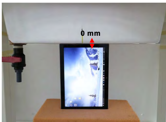
Fig.6 EUT Right side to flat phantom
