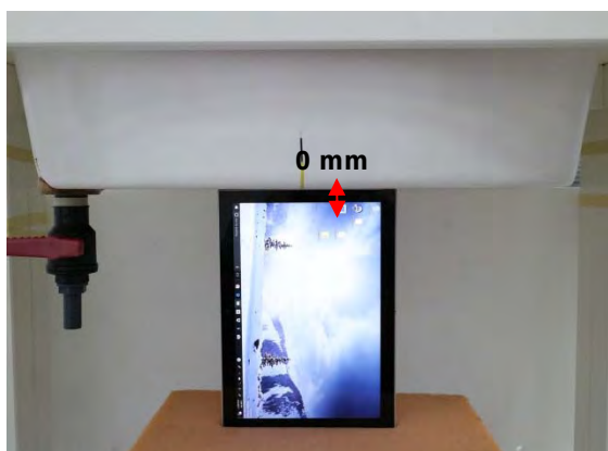
Fig.7 EUT Left side to flat phantom
