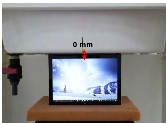
Fig.4 EUT Top side to flat phantom
