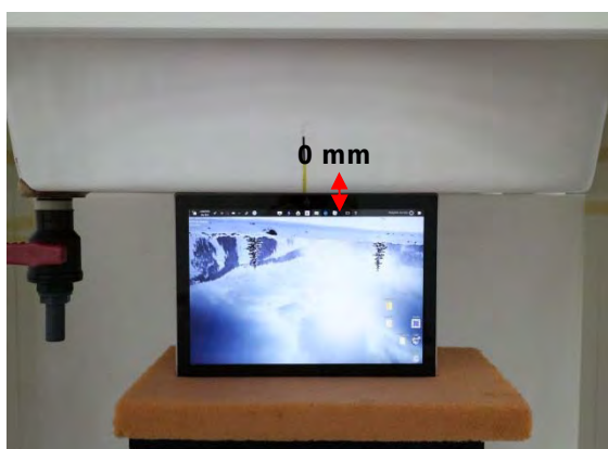
Fig.5 EUT Bottom side to flat phantom
