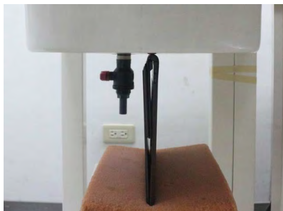
Fig.4 EUT Top side to flat phantom
