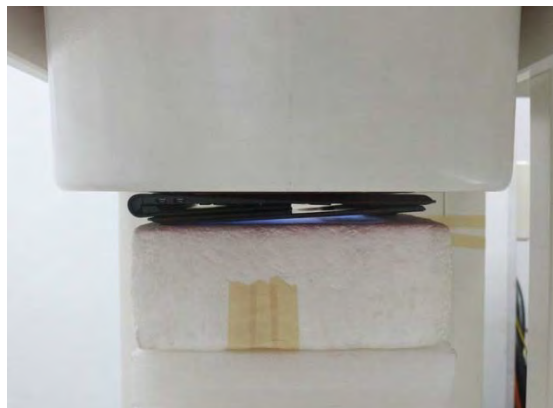
Fig.3 EUT Back side to flat phantom
