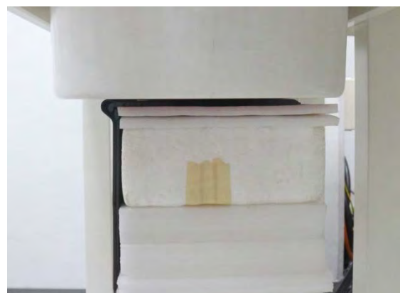
Fig.8 EUT (NB mode) Bottom side to flat phantom
