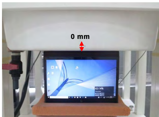
Fig.4 EUT Top side to flat phantom
