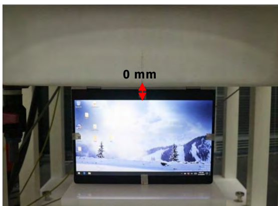
Fig.5 EUT Bottom side to flat phantom
