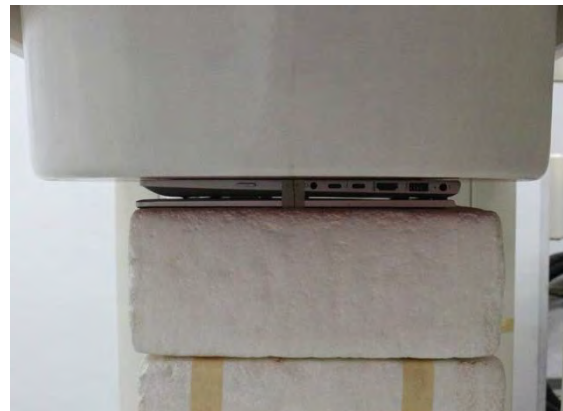
Fig.3 EUT Back side to flat phantom
