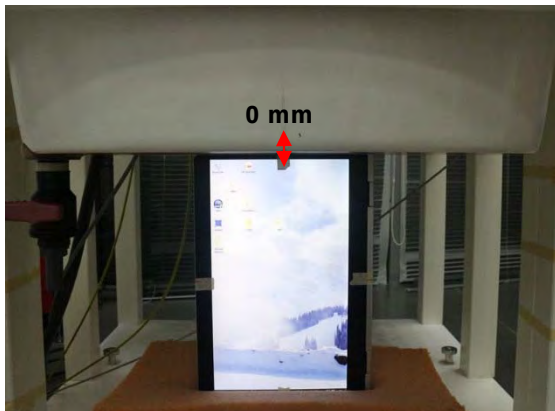
Fig.6 EUT Right side to flat phantom
