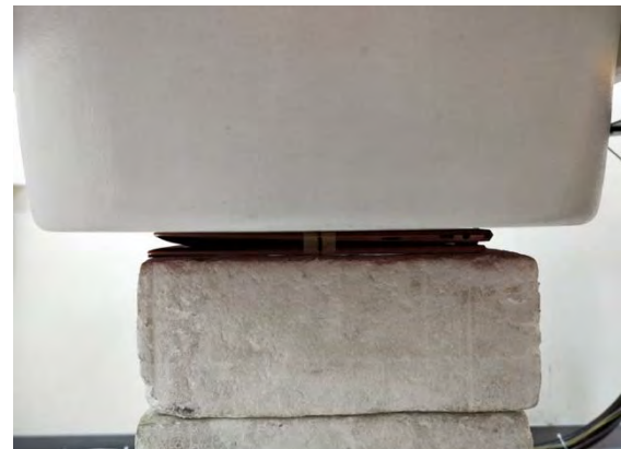
Fig.3 EUT Back side to flat phantom
