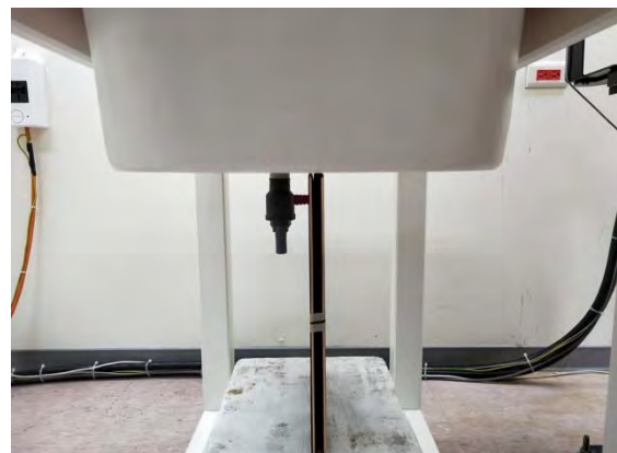
Fig.7 EUT Top side to flat phantom
