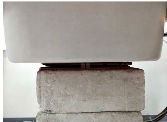
Fig.3 EUT Back side to flat phantom
