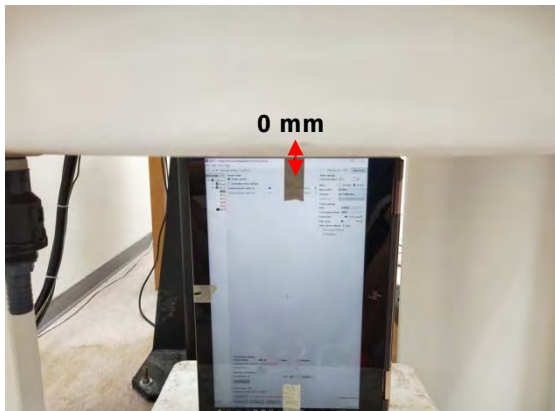
Fig.6 EUT Right side to flat phantom
