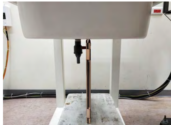
Fig.6 EUT Right side to flat phantom
