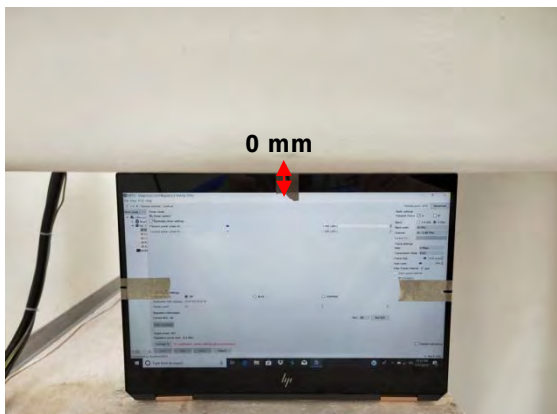
Fig.4 EUT Top side to flat phantom
