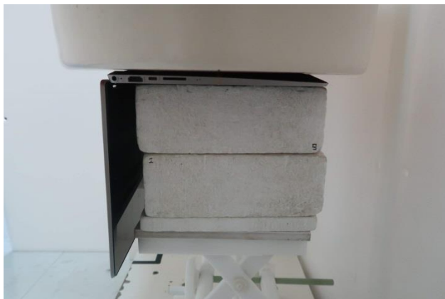
Bottom of Laptop, Test Separation 0 mm
