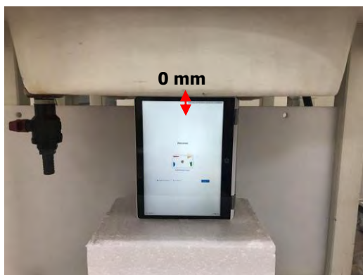
Fig.6 EUT Right side to flat phantom
