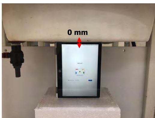
Fig.7 EUT Left side to flat phantom
