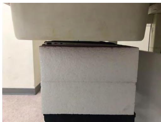
Fig.3 EUT Back side to flat phantom
