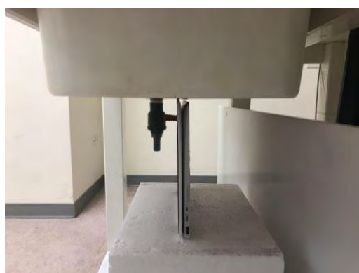
Fig.4 EUT Top side to flat phantom
