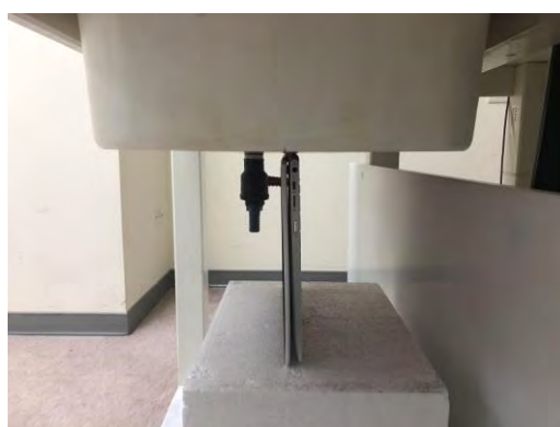
Fig.5 EUT Bottom side to flat phantom
