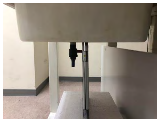
Fig.6 EUT Right side to flat phantom
