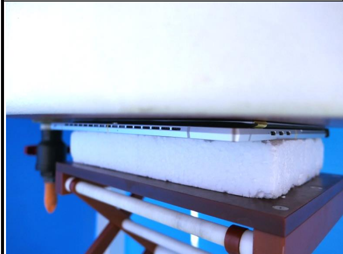
Body - Rear Face of EUT at 0 mm with Keyboard 2
