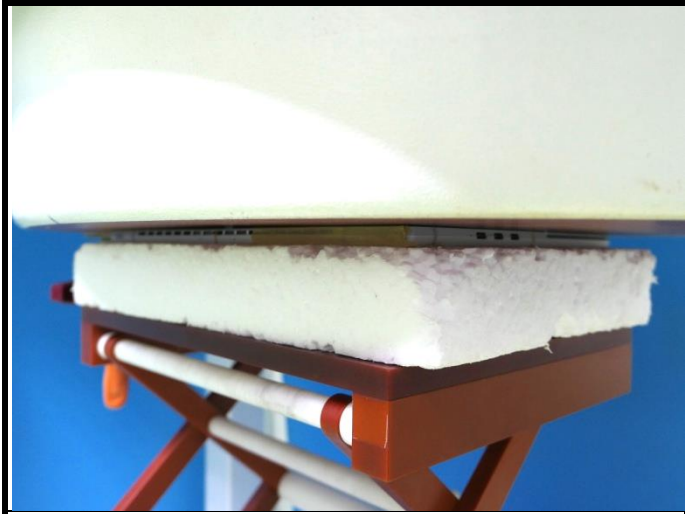
Body - Rear Face of EUT at 0 mm
