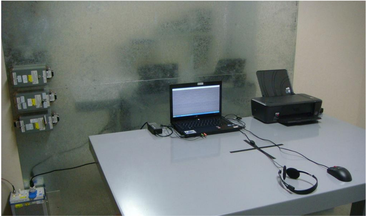
Photograph 5: Set-up for for Mains Conducted testing Back
