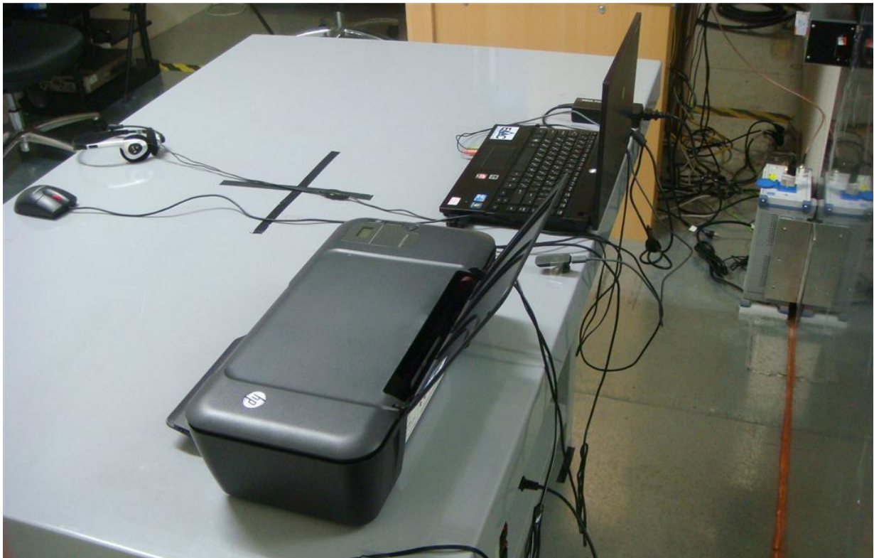
Photograph 6: Set-up for for Mains Conducted testing Front
