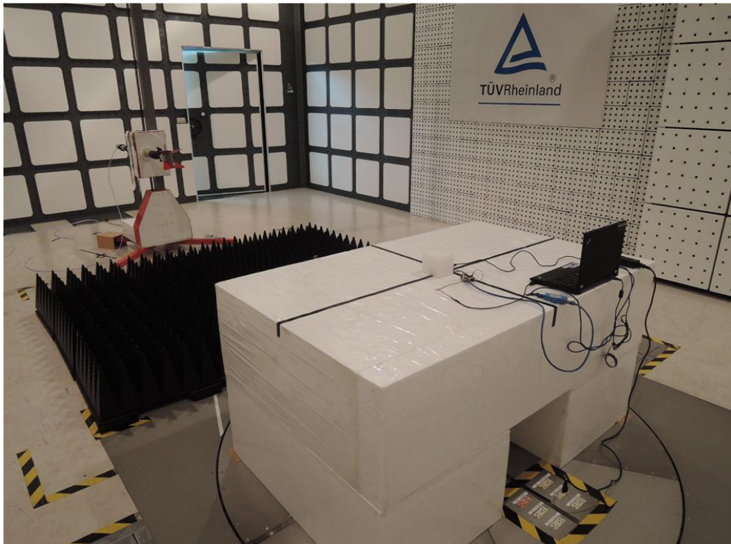
Photograph 3: Set-up for Spurious Emissions (Back View 2)
