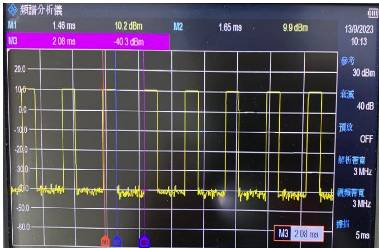
Time-domain plot for Bluetooth transmission signal
