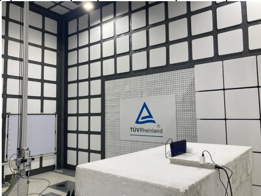
Photograph 6: Test Setup for Spurious Emissions (Back View 4)
