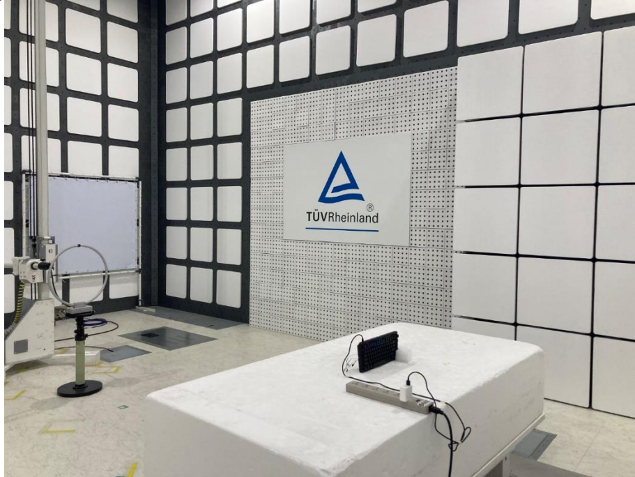
Photograph 3: Test Setup for Spurious Emissions (Back View 1)
