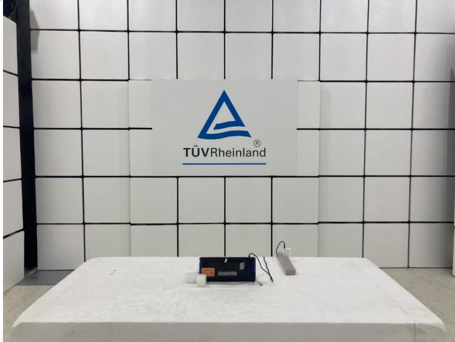
Photograph 1: Test Setup for Spurious Emissions (Front View 1)
