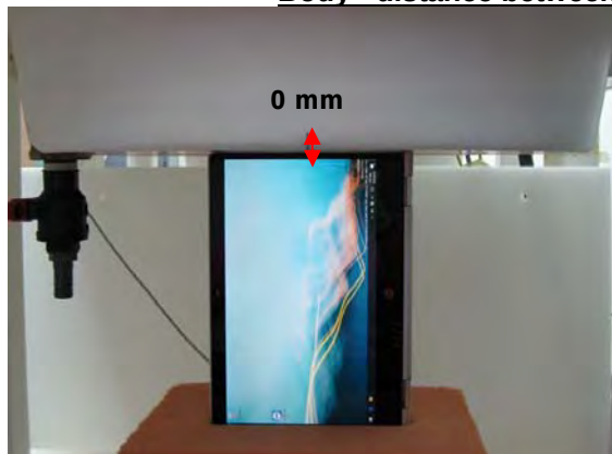
Fig.5 EUT Right side to flat phantom
