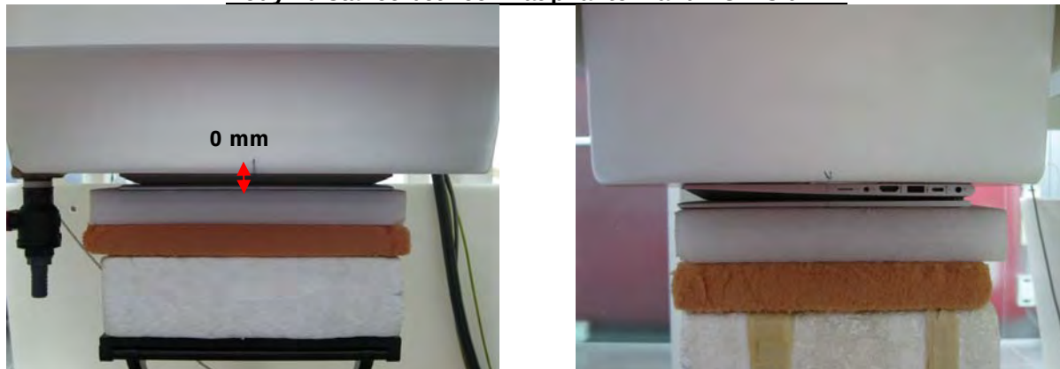
Fig.3 EUT Back side to flat phantom
