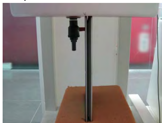
Fig.6 EUT Left side to flat phantom
