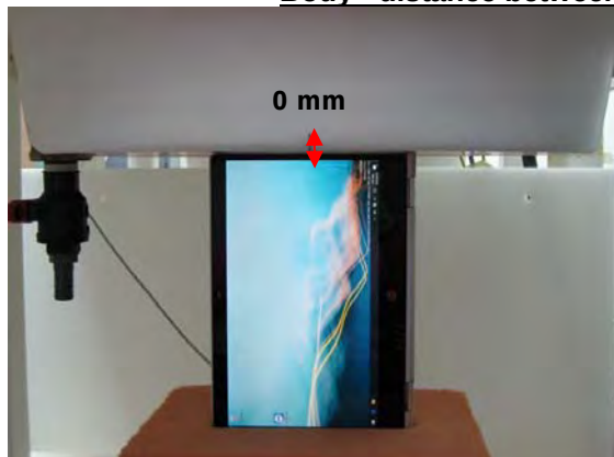
Fig.5 EUT Right side to flat phantom
