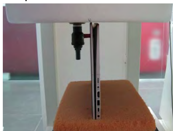
Fig.4 EUT Top side to flat phantom
