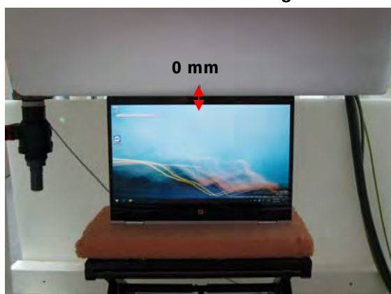
Fig.4 EUT Top side to flat phantom
