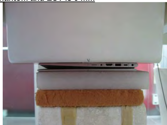
Fig.3 EUT Back side to flat phantom
