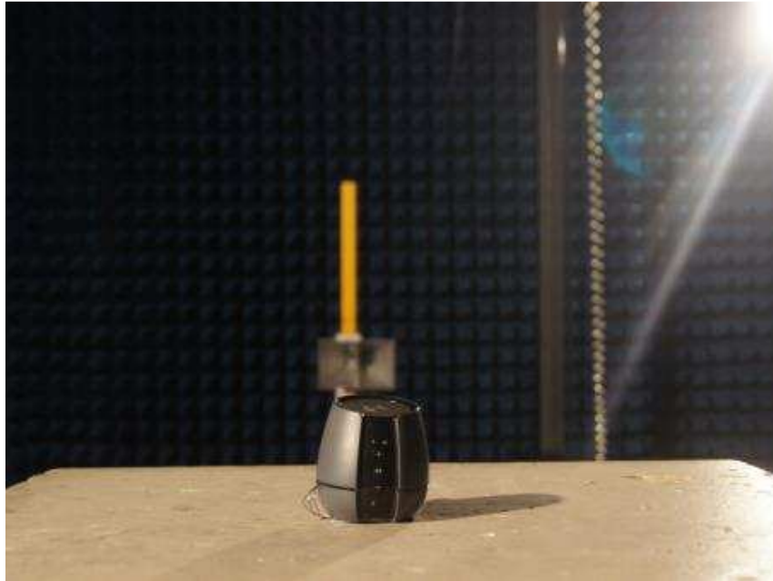
Photograph 4: Set-up for Radiated Spurious Emissions (18GHz ~ 26GHz)
