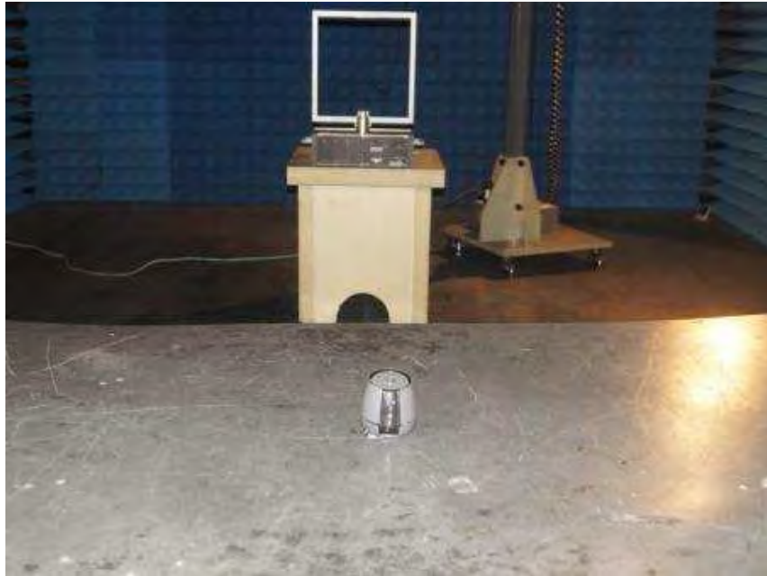
Photograph 2: Set-up for Radiated Spurious Emissions (30MHz-1GHz)
