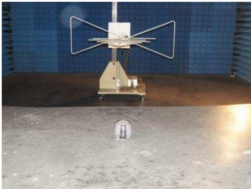
Photograph 2: Set-up for Radiated Spurious Emissions (30MHz-1GHz)
