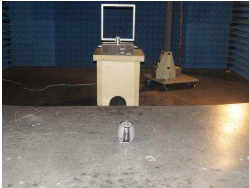
Photograph 2: Set-up for Radiated Spurious Emissions (30MHz-1GHz)
