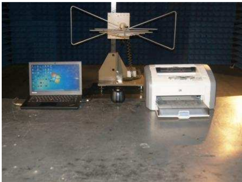
Photograph 6: Set-up for Radiated Emission (Below 1GHz)
