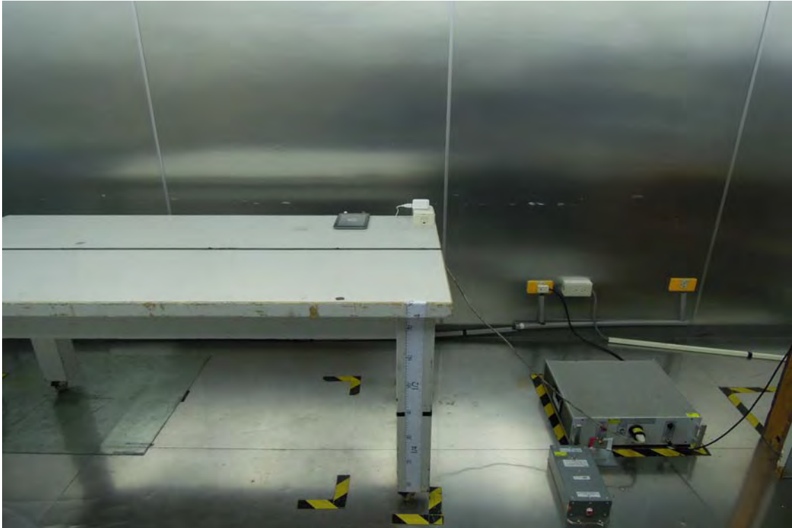
AC Power-line Conducted Emission Set up Photo
