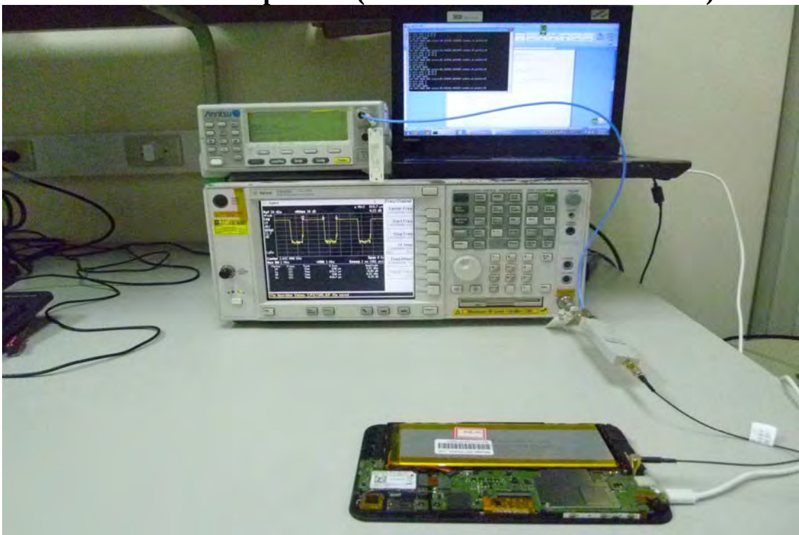
Conducted Setup Photo (Measurement at Antenna Port)
