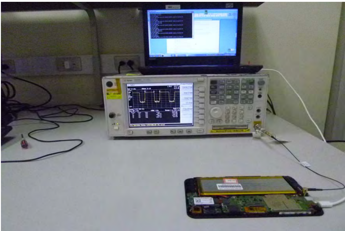
Conducted Setup Photo (Measurement at Antenna Port)
