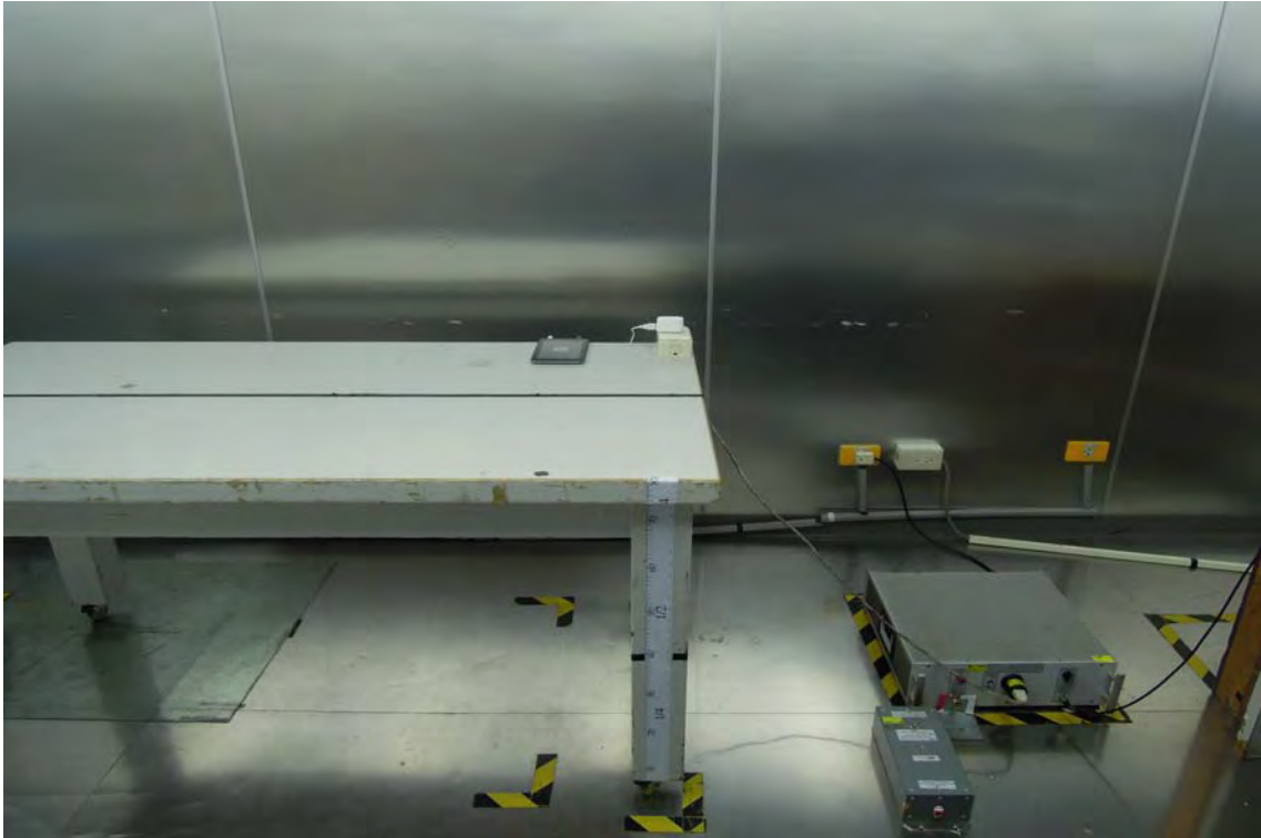
AC Power-line Conducted Emission Set up Photo
