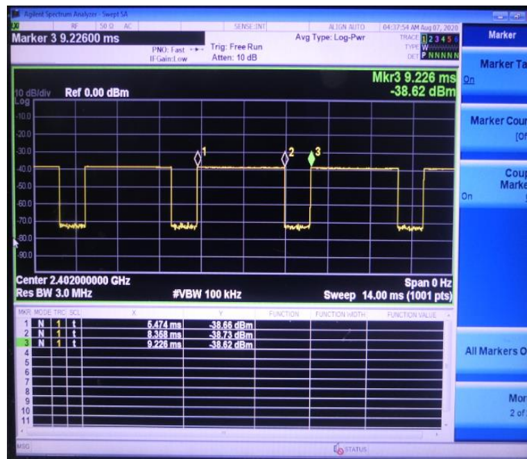
Time-domain plot for Bluetooth transmission signal
