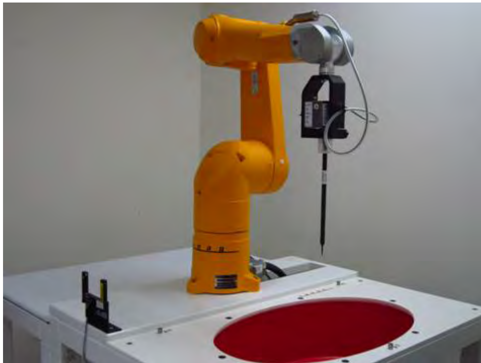
Fig.1 Photograph of the SAR measurement system
