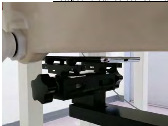
Fig.8 EUT Front side to flat phantom
