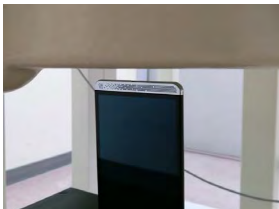
Fig.9 EUT Bottom side to flat phantom
