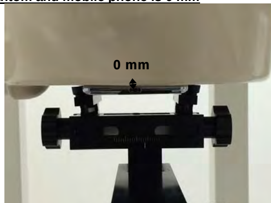
Fig.14 EUT front to flat phantom
