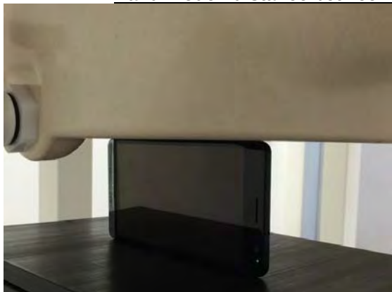
Fig.17 EUT left to flat phantom
