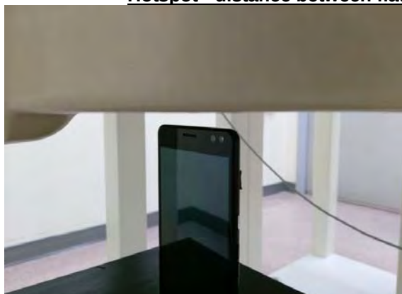
Fig.11 EUT Top side to flat phantom
