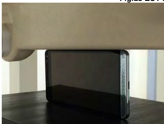
Fig.16 EUT right to flat phantom
