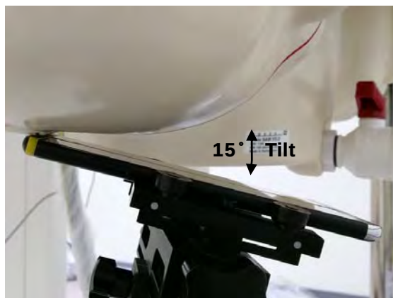
Fig.5 Right Head Section / Ear-Tilt Position(15°)
