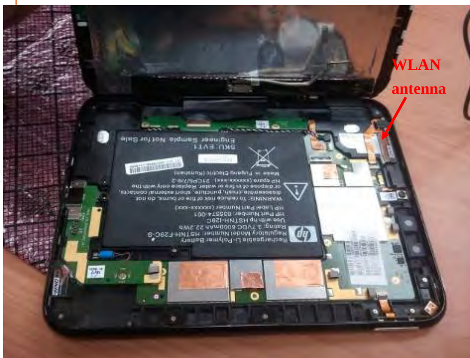
Fig.10 Antenna position of EUT
