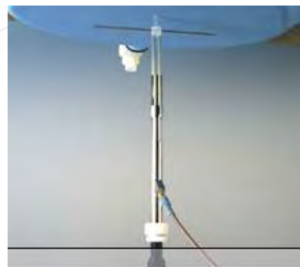
Photograph of the dipole Antenna
