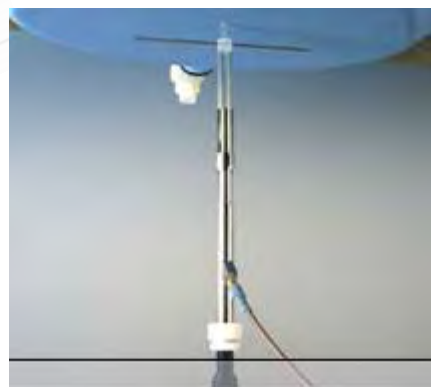
Photograph of the dipole Antenna
