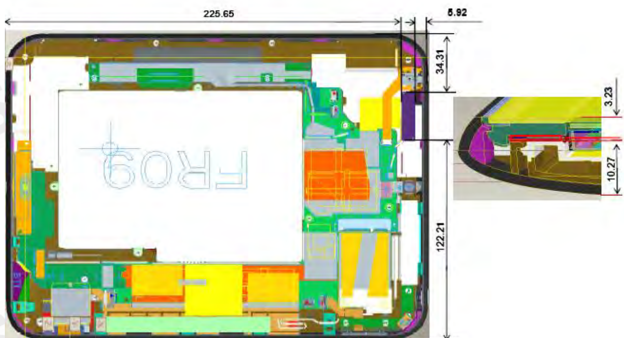
Fig.10 Antenna position &amp; distance
