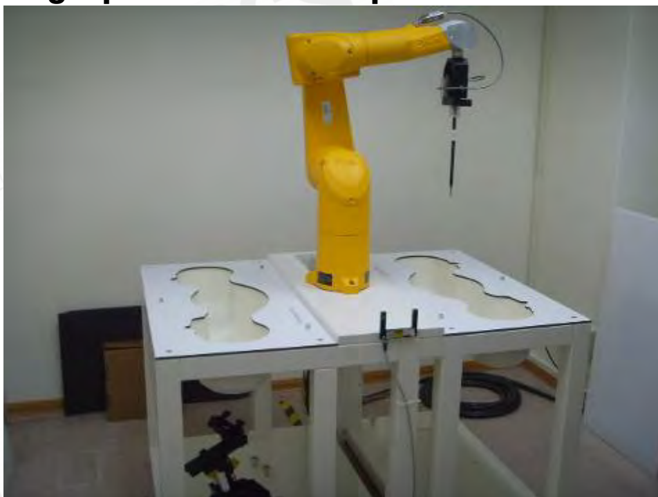
Fig.1 Photograph of the SAR measurement System
