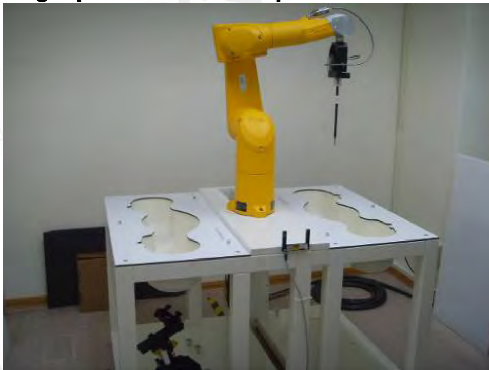
Fig.1 Photograph of the SAR measurement System
