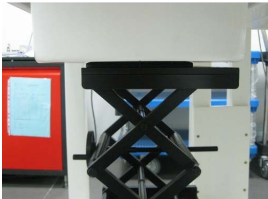
Fig.3 EUT Lap-held mode to flat phantom
