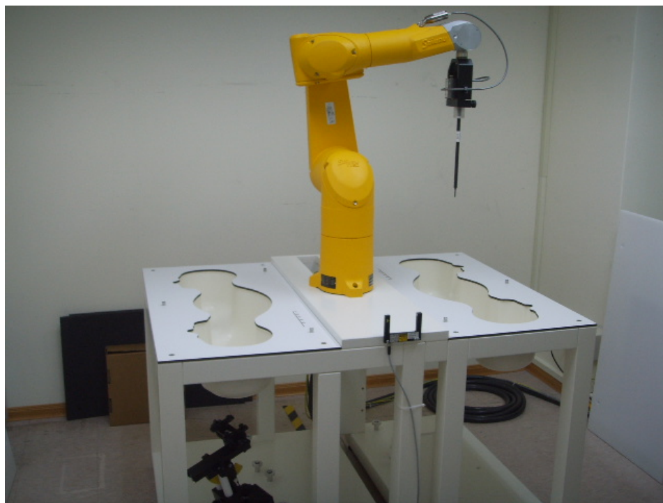
Fig.1 Photograph of the SAR measurement system
