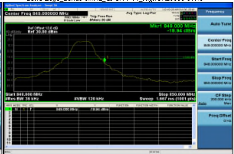
Band Edge_Band5 3MHz_QPSK 1 14_HighCH20635-847.5
