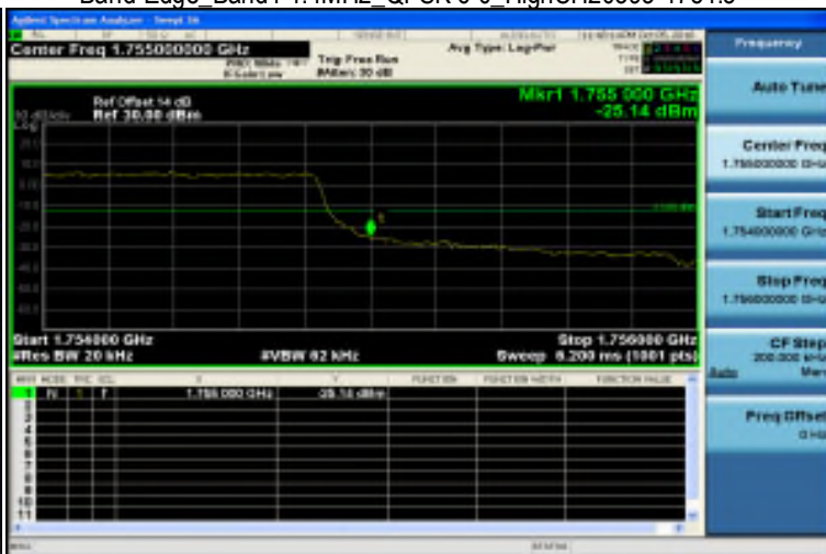
Band Edge_Band4 1.4MHz_QPSK 6 0_HighCH20393-1754.3
