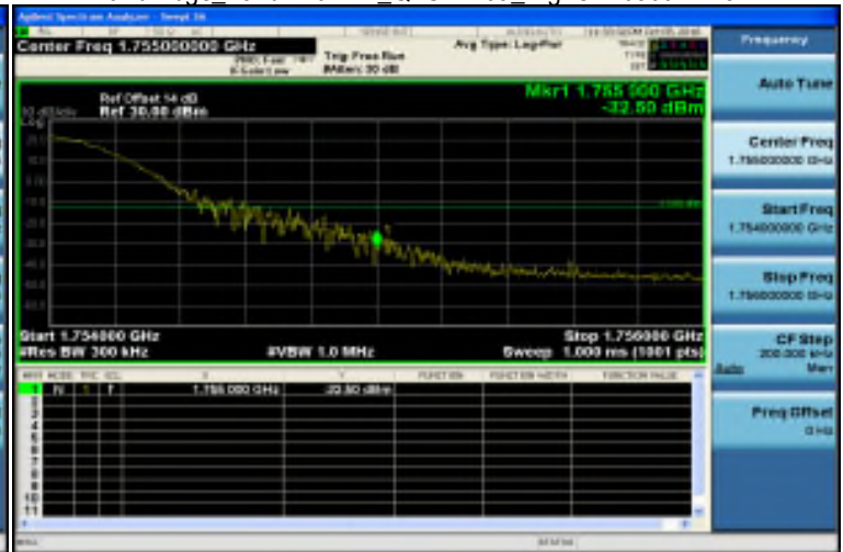
Band Edge_Band4 20MHz_QPSK 1 99_HighCH20300-1745
