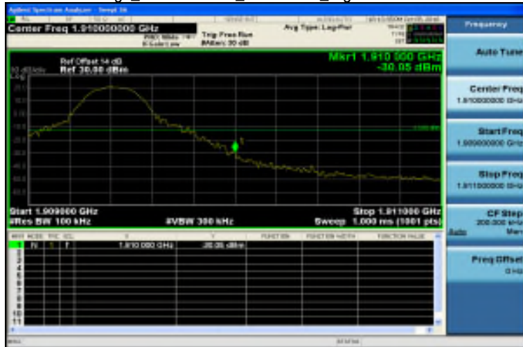
Band Edge_Band2 10MHz_QPSK 1 49_HighCH19150-1905
