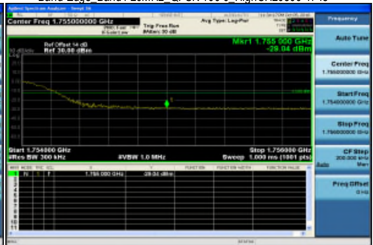
Band Edge_Band4 20MHz_QPSK 100 0_HighCH20300-1745
