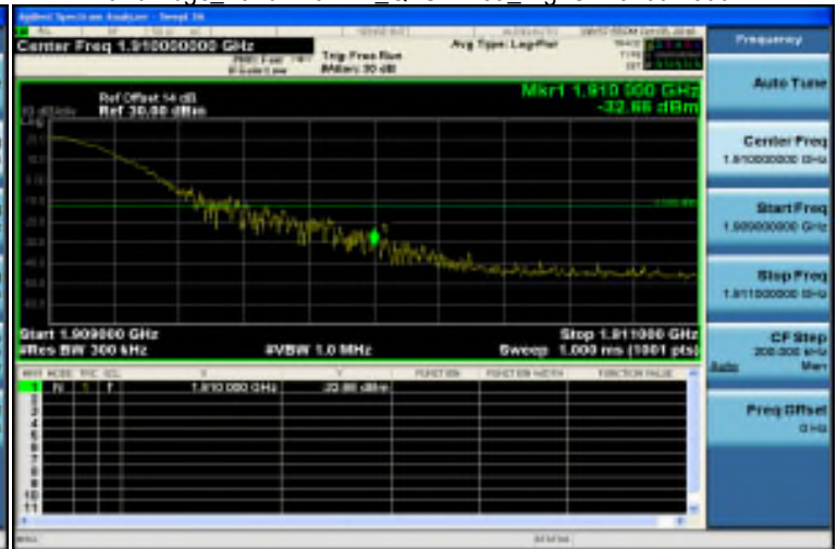
Band Edge_Band2 20MHz_QPSK 1 99_HighCH19100-1900
