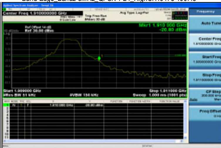
Band Edge_Band2 5MHz_QPSK 1 24_HighCH19175-1907.5
