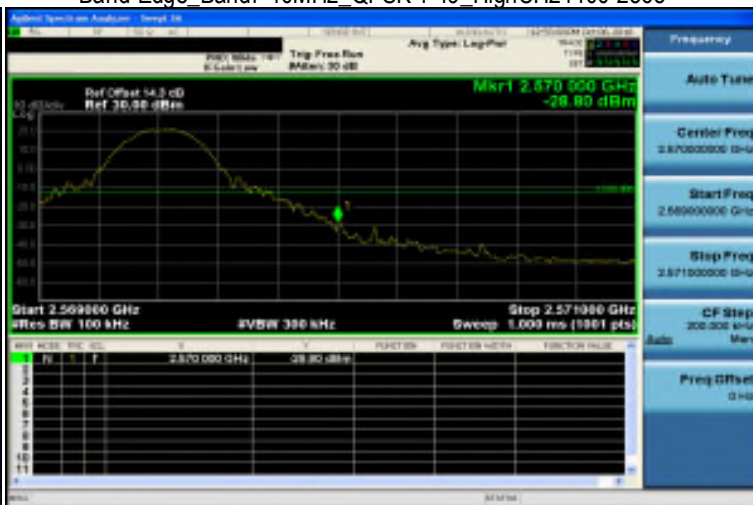
Band Edge_Band7 10MHz_QPSK 1 49_HighCH21400-2565
