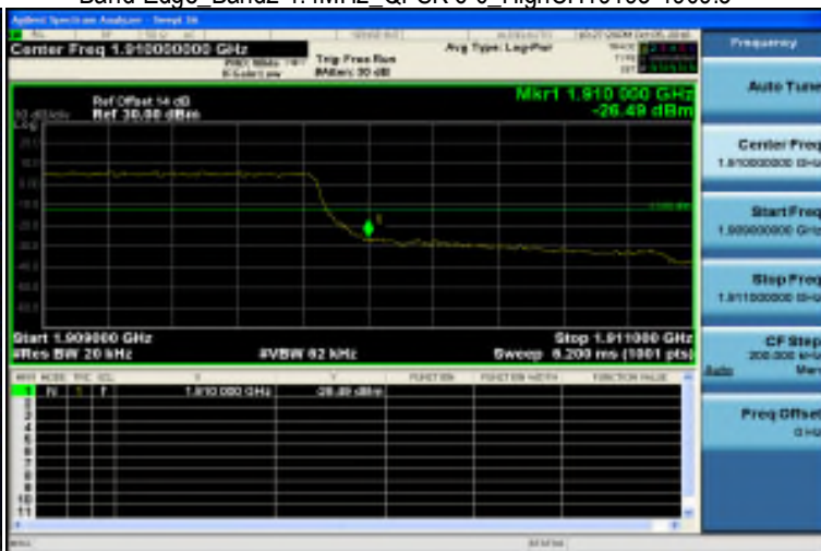
Band Edge_Band2 1.4MHz_QPSK 6 0_HighCH19193-1909.3
