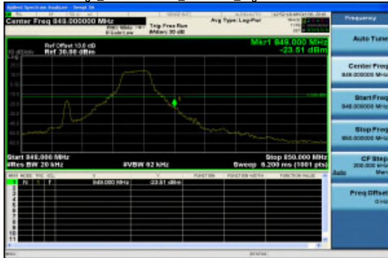
Band Edge_Band5 1.4MHz_QPSK 1 5_HighCH20643-848.3
