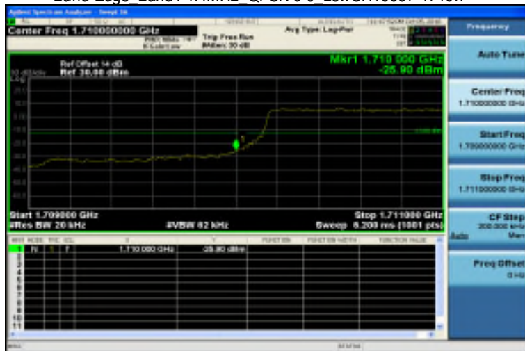
Band Edge_Band4 1.4MHz_QPSK 6 0_LowCH19957-1710.7
