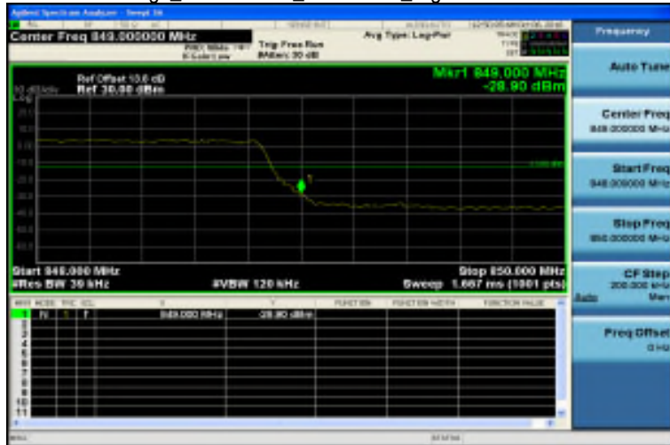
Band Edge_Band5 3MHz_QPSK 15 0_HighCH20635-847.5
