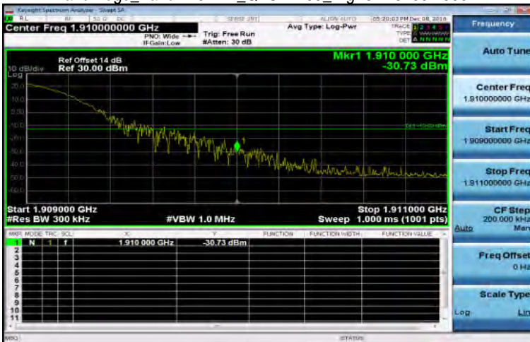
Band Edge_Band2 20MHz_QPSK 1 99_HighCH19100-1900
