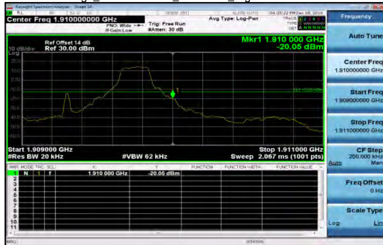
Band Edge_Band2 1.4MHz_QPSK 1 5_HighCH19193-1909.3
