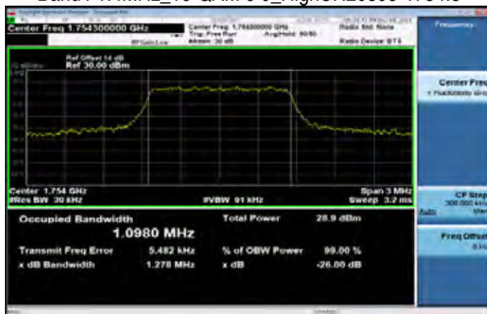
Band4 1.4MHz_16-QAM 6 0_HighCH20393-1754.3
