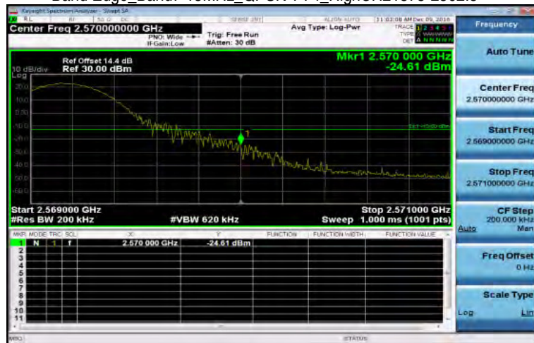
Band Edge_Band7 15MHz_QPSK 1 74_HighCH21375-2562.5
