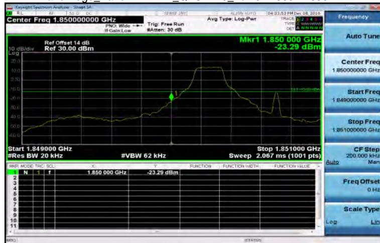
Band Edge_Band2 1.4MHz_QPSK 1 0_LowCH18607-1850.7
