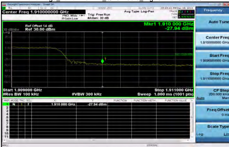
Band Edge_Band2 10MHz_QPSK 50 0_HighCH19150-1905
