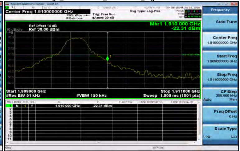
Band Edge_Band2 5MHz_QPSK 1 24_HighCH19175-1907.5
