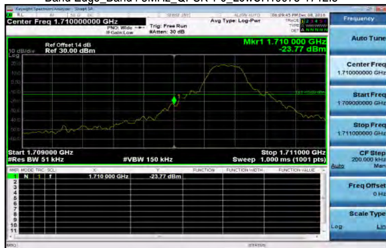
Band Edge_Band4 5MHz_QPSK 1 0_LowCH19975-1712.5
