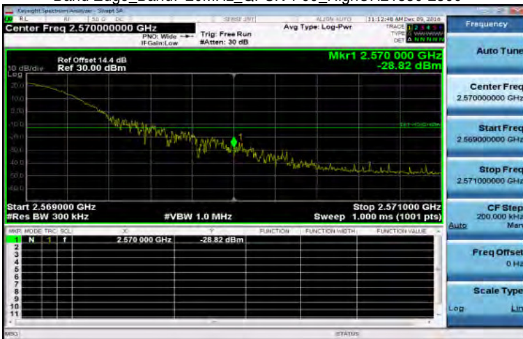
Band Edge_Band7 20MHz_QPSK 1 99_HighCH21350-2560
