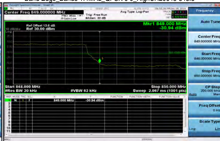
Band Edge_Band5 1.4MHz_QPSK 6 0_HighCH20643-848.3
