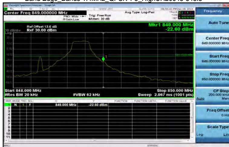
Band Edge_Band5 1.4MHz_QPSK 1 5_HighCH20643-848.3
