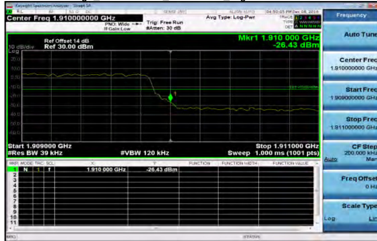
Band Edge_Band2 3MHz_QPSK 15 0_HighCH19185-1908.5
