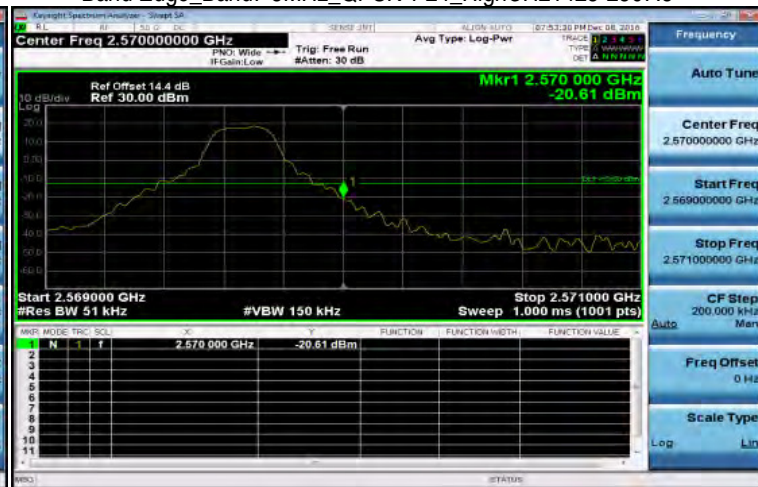
Band Edge_Band7 5MHz_QPSK 1 24_HighCH21425-2567.5
