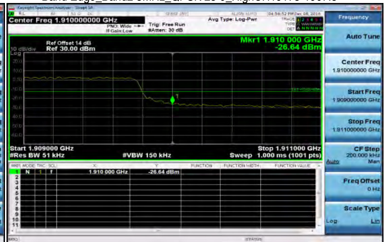
Band Edge_Band2 5MHz_QPSK 25 0_HighCH19175-1907.5
