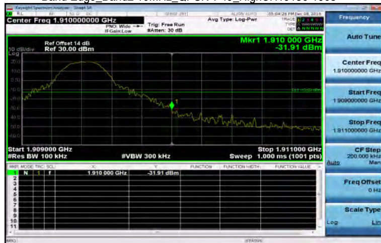
Band Edge_Band2 10MHz_QPSK 1 49_HighCH19150-1905
