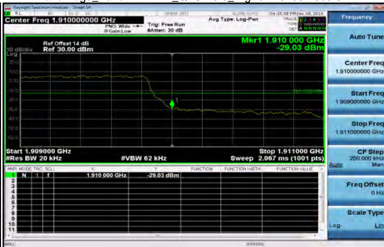
Band Edge_Band2 1.4MHz_QPSK 6 0_HighCH19193-1909.3
