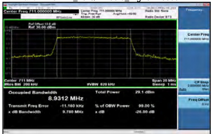
Band17 10MHz_16-QAM 50 0_HighCH23800-711
