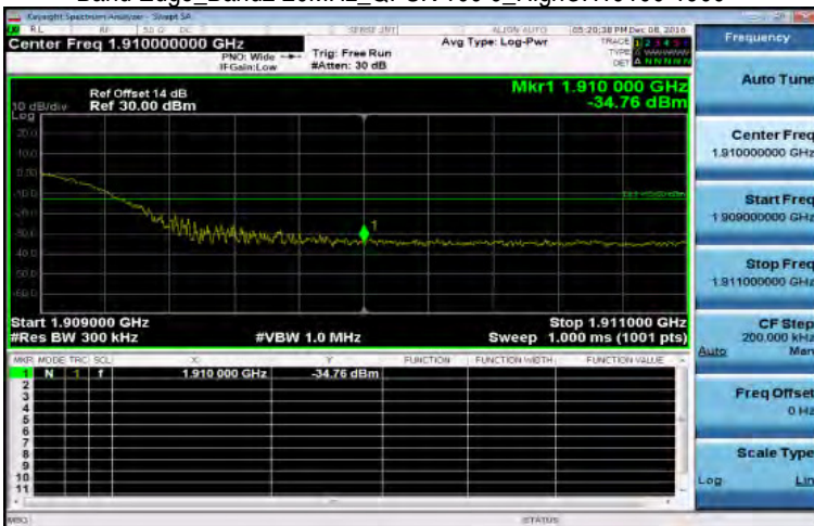
Band Edge_Band2 20MHz_QPSK 100 0_HighCH19100-1900
