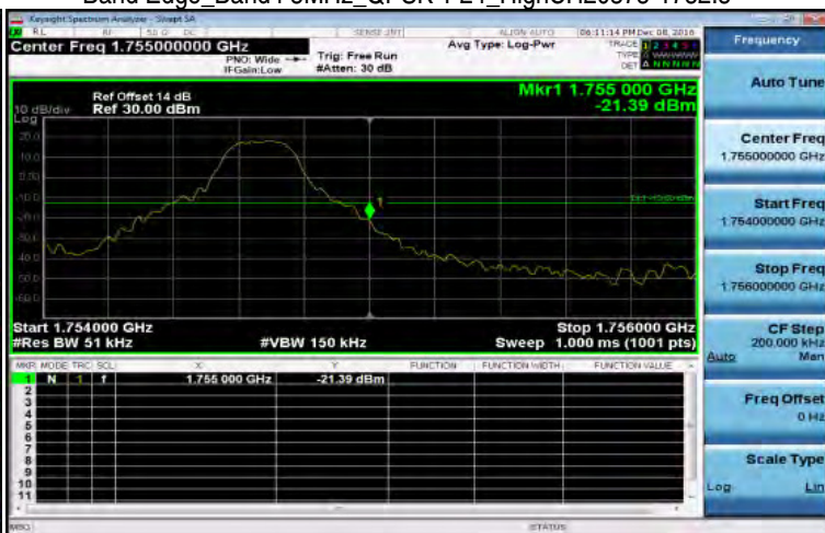
Band Edge_Band4 5MHz_QPSK 1 24_HighCH20375-1752.5
