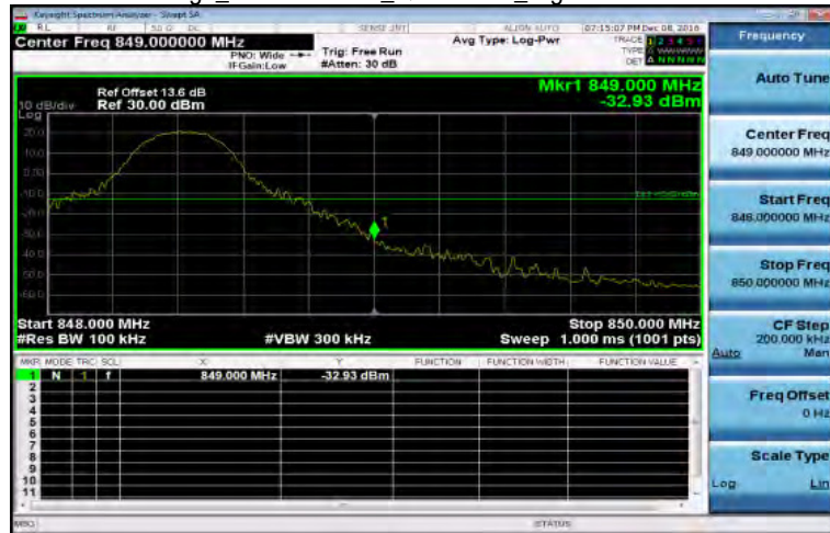
Band Edge_Band5 10MHz_QPSK 1 49_HighCH20600-844
