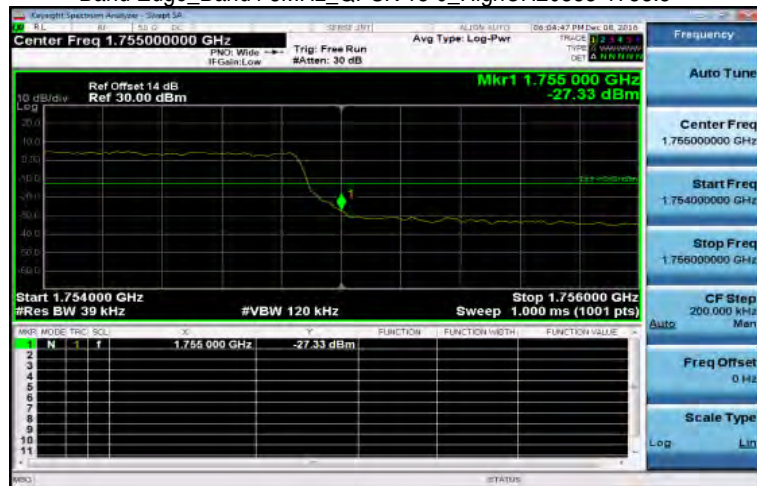
Band Edge_Band4 3MHz_QPSK 15 0_HighCH20385-1753.5
