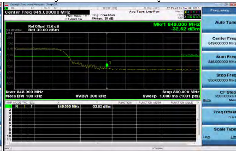
Band Edge_Band5 10MHz_QPSK 50 0_HighCH20600-844
