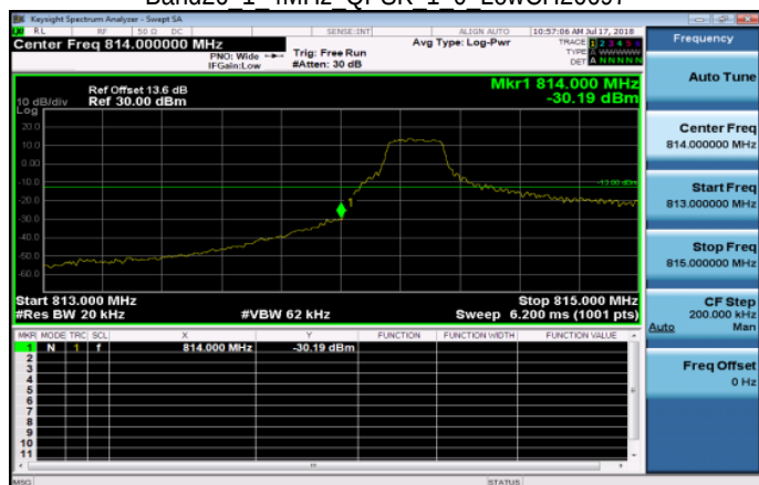
Band26 1 4MHz QPSK 1 5 HighCH26783
