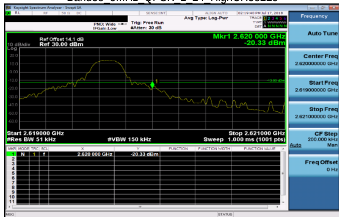
Band38 5MHz QPSK 1 24 HighCH38225
