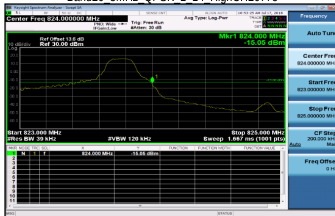
Band26 3MHz QPSK 1 14 HighCH26775
