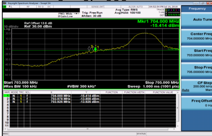
Band17 10MHz QPSK 1 49 HighCH23800-711
