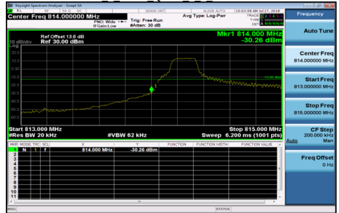
Band26 1 4MHz QPSK 1 5 HighCH27033
