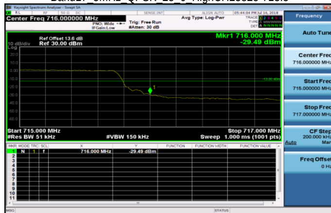
Band17 5MHz QPSK 25 0 HighCH23825-713.5
