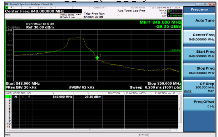
Band26 1 4MHz QPSK 1 5 HighCH27033
