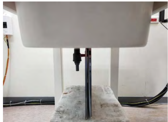
Fig.5 EUT Bottom side to flat phantom
