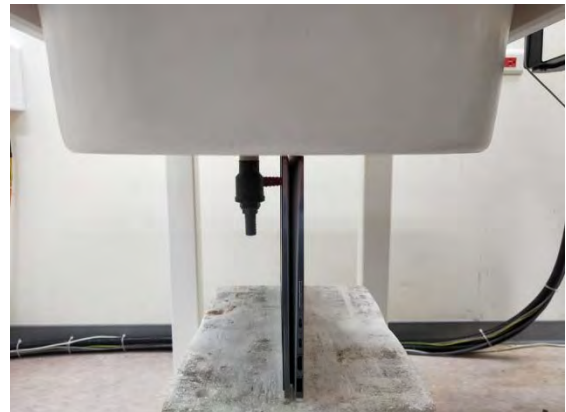
Fig.4 EUT Top side to flat phantom
