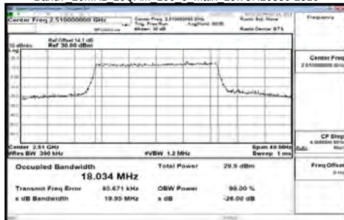
Band7 20MHz 16QAM 100 0 Main LowCH20850-2510
