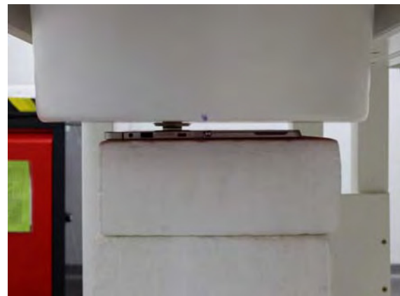
Fig.4 EUT Back side (10mm) to flat phantom
